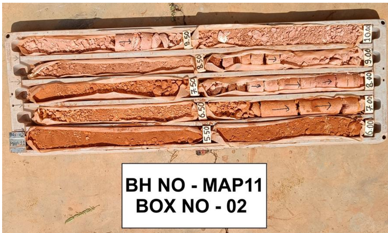
Photograph No.7: Core Photograph of MAP-11 showing Clay intercepted between 6.00 to 10.00m
