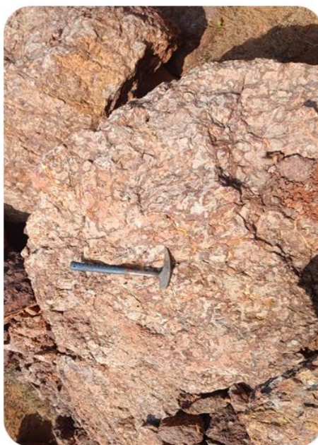
Photo 4: Pisolitic bauxite in the block
