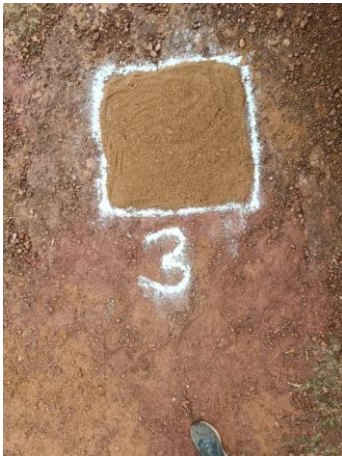
Photograph showing the Pits excavated for calculation of Bulk density
