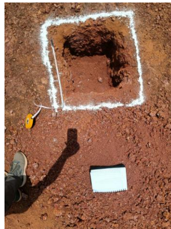
Photograph showing the Pits excavated for calculation of Bulk density
