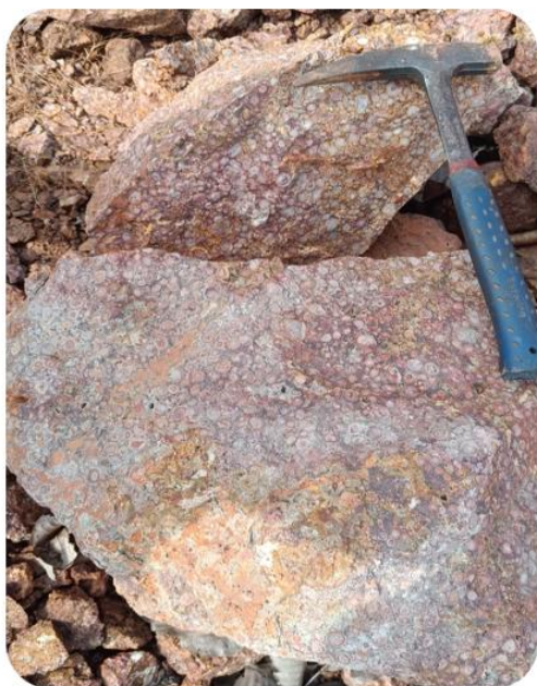
Photo 3: Iron Intrusion in Aluminous laterite and spherical nodules of iron
