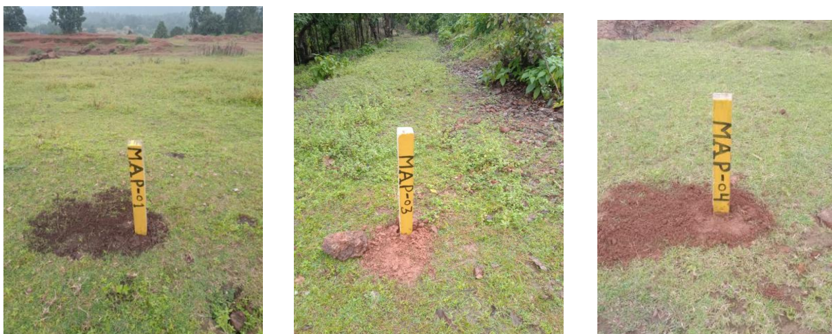
Photograph No.9 to 11: Pillars constructed on boreholes drilled in Anvarapat block by MECL.
